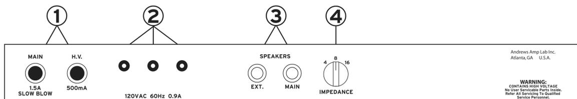
**1. FUSES** – Always use correctly rated fuses. The MAIN fuse should be replaced only with a 1.5 Amp “Slow Blow” 250 volt type. The H.V. fuse should be replaced only with a 500mA (1/2 Amp) fast acting 250V type. Always unplug the AC cord before changing fuses. When installing a new fuse, first insert it into the cap of the fuse holder, then while holding only the cap, insert the fuse into the holder, push in and turn clockwise to lock the cap and fuse in place.
